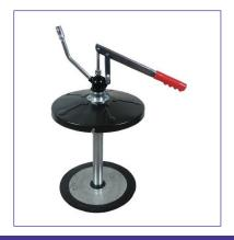
The 20kg grease pump is suitable for bulk filling of manual or electric hand grease guns. With a durable cast aluminium alloy pump outlet body, it allows for the fast reload of grease guns, taking less than a minute. The nipple allows bulk fill to valve with diameters of 9mm and 12.5mm. Comes standard with a Rubber follower plate.
